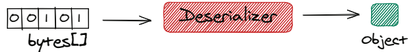
Figure 3.2 The serializer and deserializer are agnostic of the producer and consumer and perform the expected action when executing the serialize and deserialize methods.
