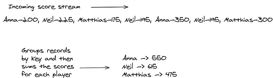
Figure 7.2 Grouping the scores by player-id ensures we only sum the scores for the individual players.
